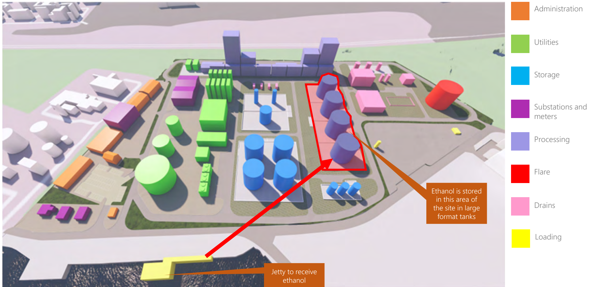
Figure 59 – Receipt of Ethanol feedstock and on-site storage. Feedstocks and products from the plant will pass to the jetty via below ground pipeworks.
