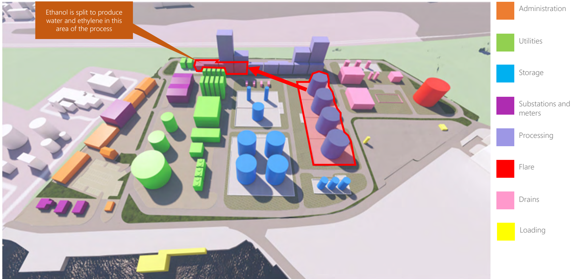
Figure 61 – Ethanol is de-hydrated and ethylene separated
