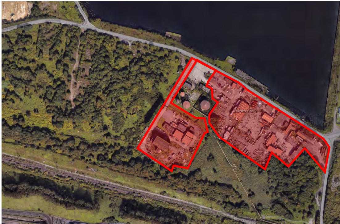
Figure 87 (Left) – Area of building to be demolished to make additional construction laydown space. The extent of demolition will be to ground level only. Where possible any masonry or concrete materials will be crushed and re-used as hardcore surfacing to the laydown area. On complete the area will be left as a hardcore finish for pioneer species to recolonise.
