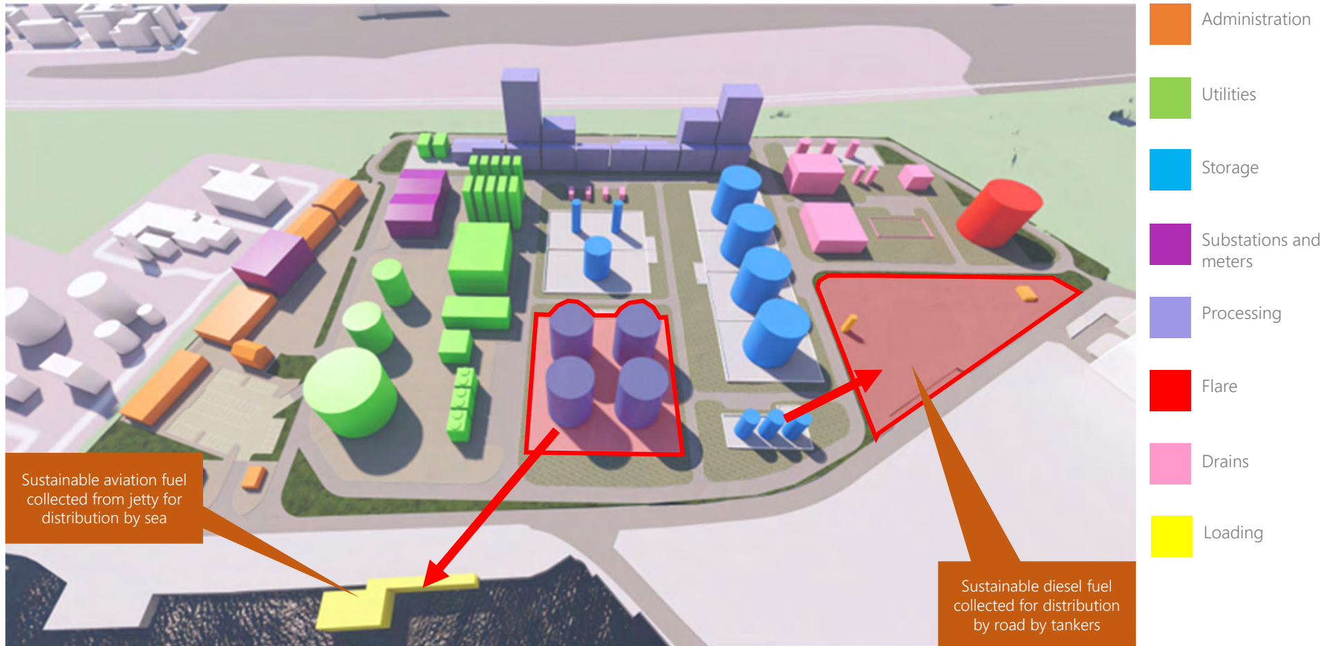
Figure 64 – Distribution of finished products. Products will be moved around the site via pipe runs that are not shown in this diagram for clarity. For details of pipe runs refer to the architectural drawings.
